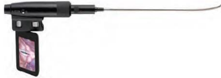
Fig. 1.16. The Clarus Video System incorporates a curved stylet containing a CMOS chip video camera surrounding by a malleable but rigid protective metal sheath. Images are displayed on a video screen attached to the handle. The screen can swivel for optimal viewing as the stylet is inserted into the mouth. (Courtesy Clarus Medical, Minneapolis.)
